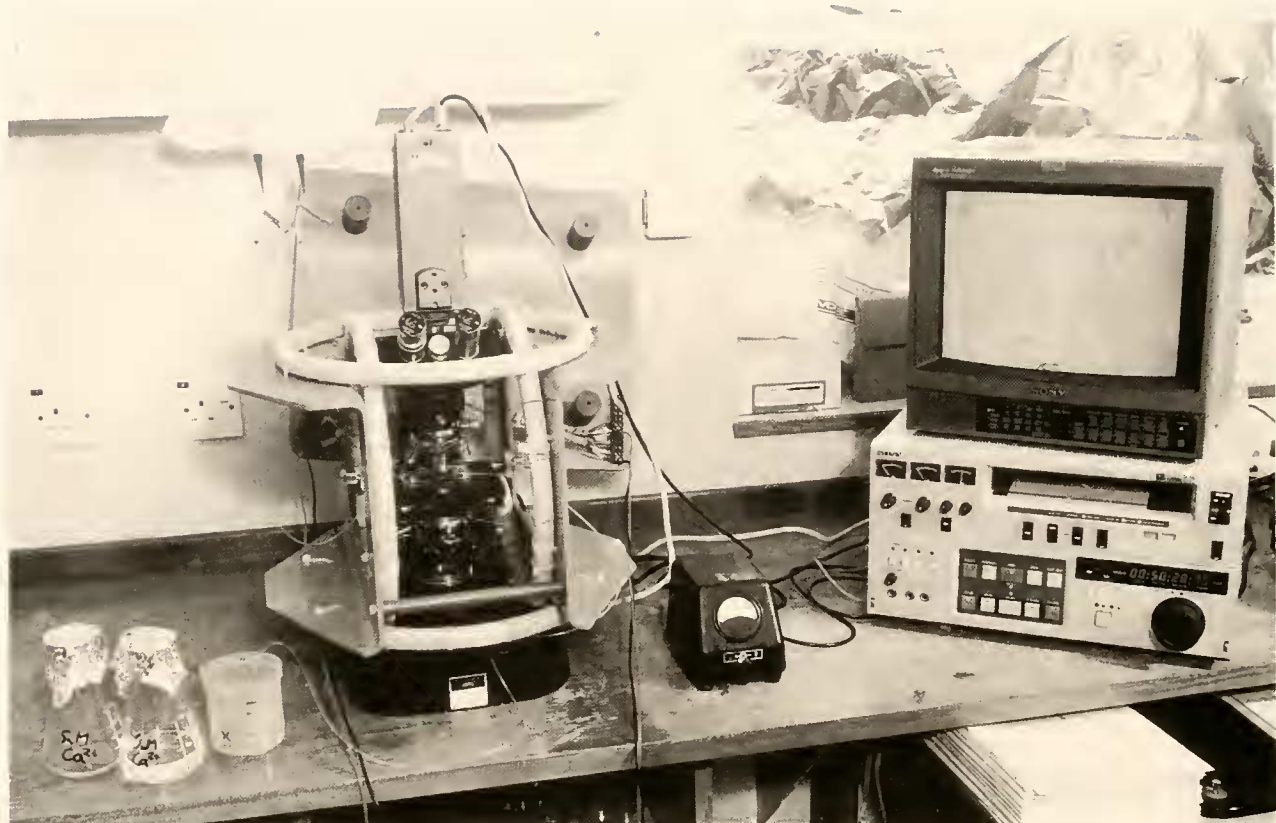
Figure 3. Equipment used in perfusion experiments. Near-Helmholtz coils arranged around microscope stage. Video display of diatoms in perfusion chamber.
